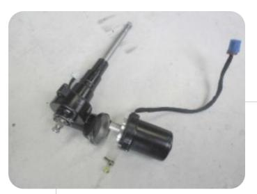
**Step 13.** Remove the electric motor from the EZ unit.
