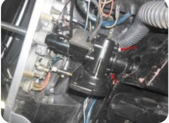
Step 18. Install the output tube back on the EZ unit.
