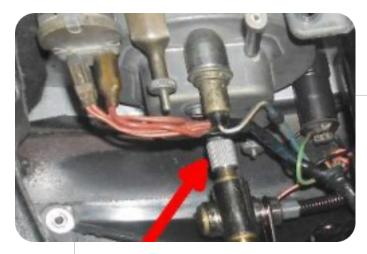
Step 7. Install the speed sensor between the cable and speedometer.
