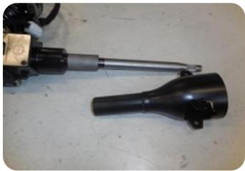
**Step 11.** Disassemble the input tube from the EZ unit.
